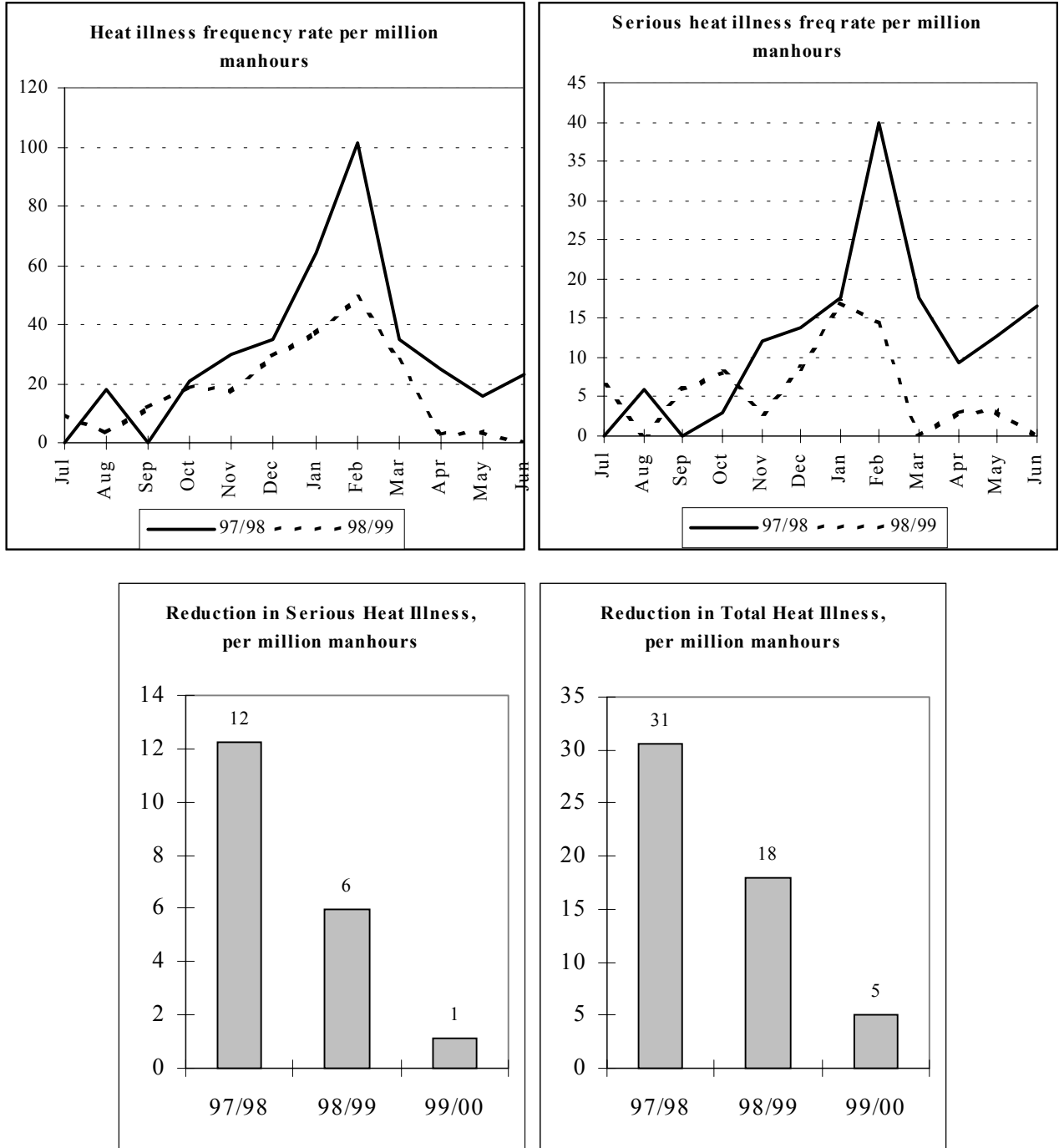
Figure 2 Reduction in heat illness at Mount Isa, before and after changes to working in heat protocols and elimination of six-hour shifts. Serious heat illness is defined arbitrarily as symptoms including vomiting or worse.
